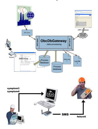
OpcDbGateway can accumulate current data from sensors of technological devices through OPC servers, evaluate them, store processed information into a process database and initialize sending of SMS messages to the maintenance employees. The service can be initialized also on elapsing of a defined time period or under other condition
