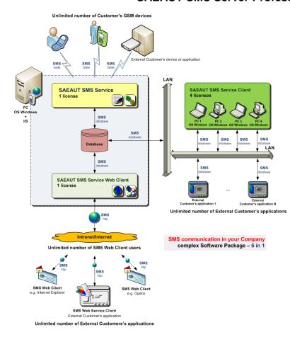
The software bundle SAEAUT SMS Server Professional is budget priced solution consisting of SAEAUT SMS Service (1 licence), SAEAUT SMS Service Client (4 licences) SAEAUT SMS Service Web Client (1 licence).
