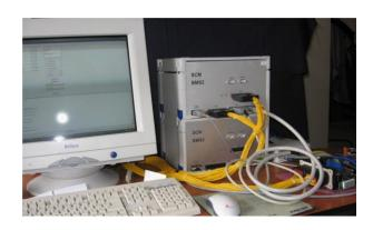
Computer controlled test equipment for automatic testing of complex microcomputer modules and logging of results into database or text files.
