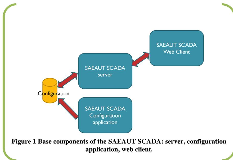
**Figure 1 Base components of the SAEAUT SCADA: server, configuration application, web client.**
